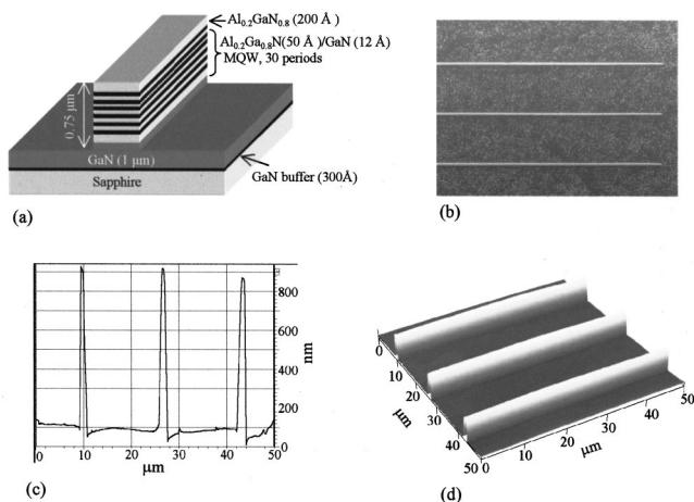
FIG. 1. (a) Schematic diagram showing the waveguide structure. (b) SEM image of the waveguide sample. The spacing between the waveguides is 15  $\mu\text{m}$ . (c), (d) AFM images of the waveguides.
