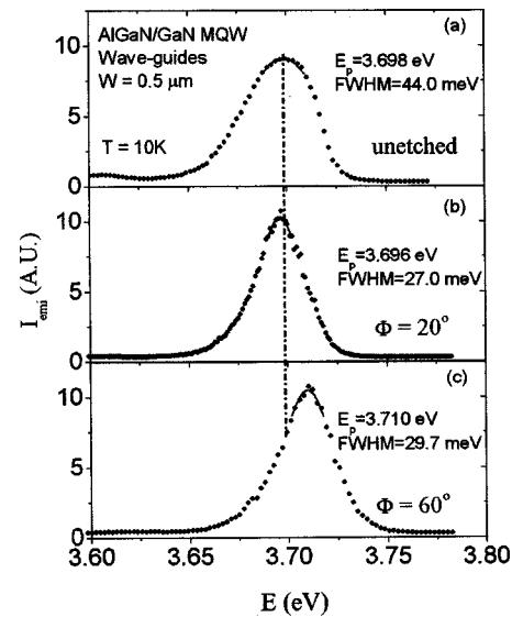
FIG. 2. Low temperature (10 K) continuous wave PL spectra from AlGaN/GaN MQW waveguides of different line orientations. For clarity, we only show (a) the PL spectrum from an unetched portion of the sample and the PL spectra from waveguides oriented at (b)  $20^\circ$  and (c)  $60^\circ$ .
