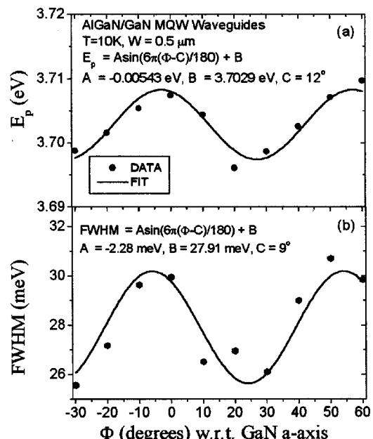
FIG. 3. Variation of (a) the spectral peak positions ( $E_p$ ) and (b) FWHM of the PL emission line at 10 K. The solid line is the sinusoidal fit of the data with six fold symmetry of the hexagonal structure.
