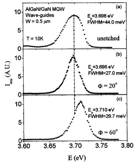
FIG. 2. Low temperature (10 K) continuous wave PL spectra from AlGaIn/GaN MQW waveguides of different line orientations. For clarity, we only show (a) the PL spectrum from an unetched portion of the sample and the PL spectra from waveguides oriented at (b) 20° and (c) 60°.
