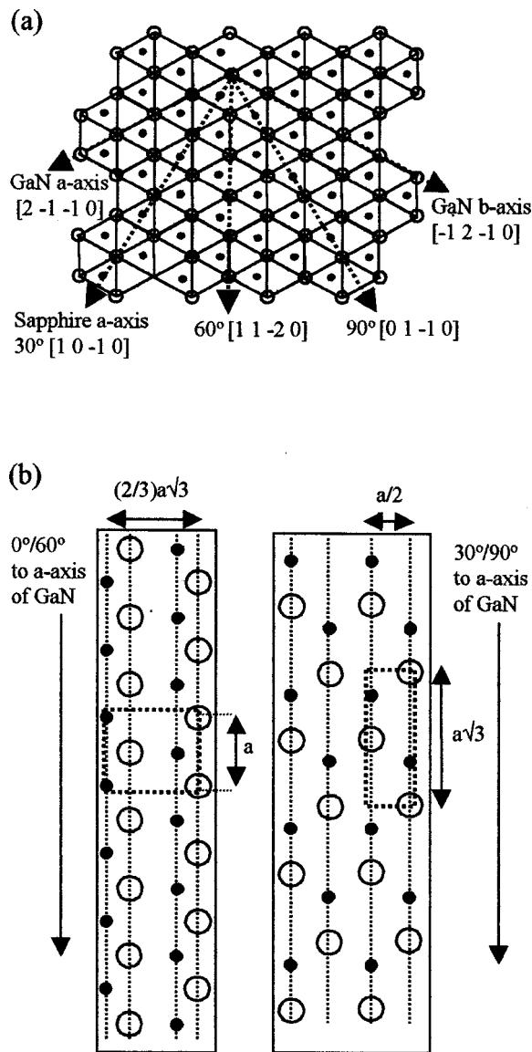
FIG. 4. (a) Crystal arrangement of  $\text{Ga}^{3+}$  (●) and  $\text{N}^{3-}$  (○) ions in a GaN hexagonal crystal structure. (b) detailed arrangements of the ions along the directions parallel to  $0^\circ/60^\circ$  (left) and  $30^\circ/90^\circ$  (right) relative to the *a* axis of the GaN crystal.
